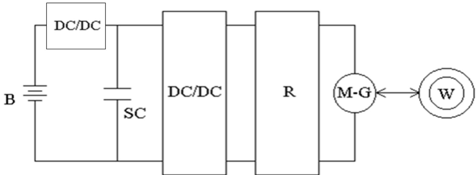
Scheme of electrical drive vehicle with supercapacitor with possibility for using breaking energy; B – one-way voltage source, SC – supercapacitor; DC/DC – direct voltage converter; R – regulator; M-G – engine – generator (depending on working regime; W – drive wheels
