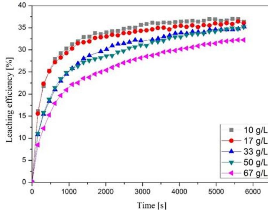
Fig. 2 Effect pulp density on the leaching of waste  $\text{LiCoO}_2$
