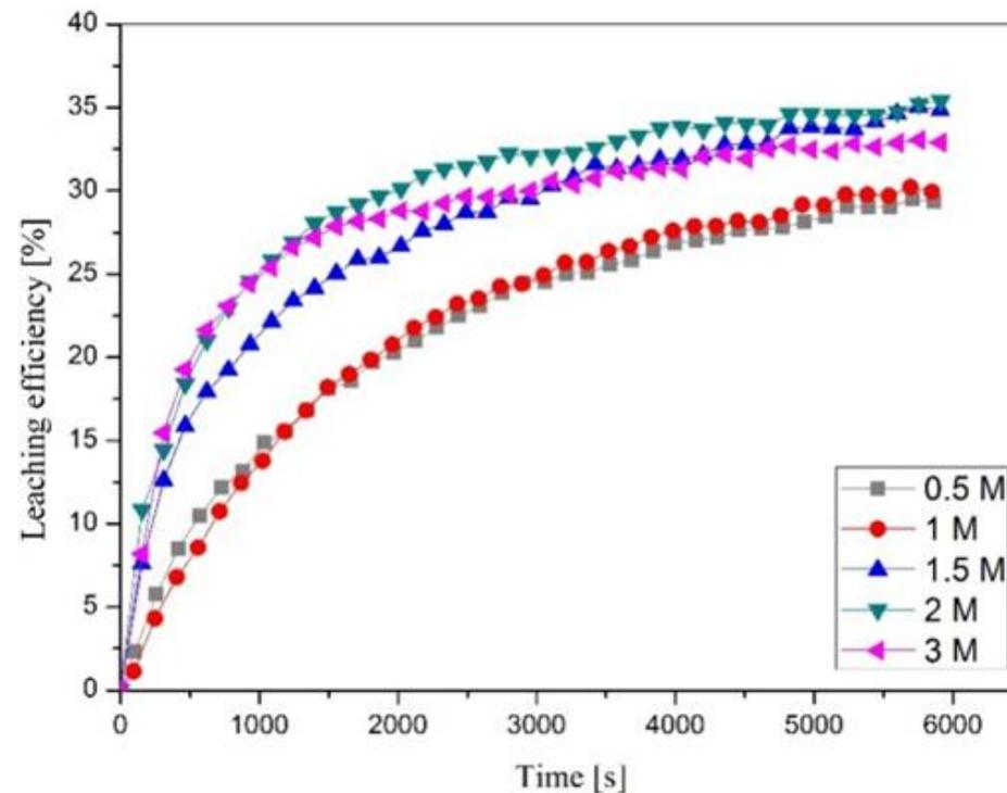
Fig.1 Effect of H<sub>2</sub>SO<sub>4</sub> concentration on the leaching of waste LiCoO<sub>2</sub>
