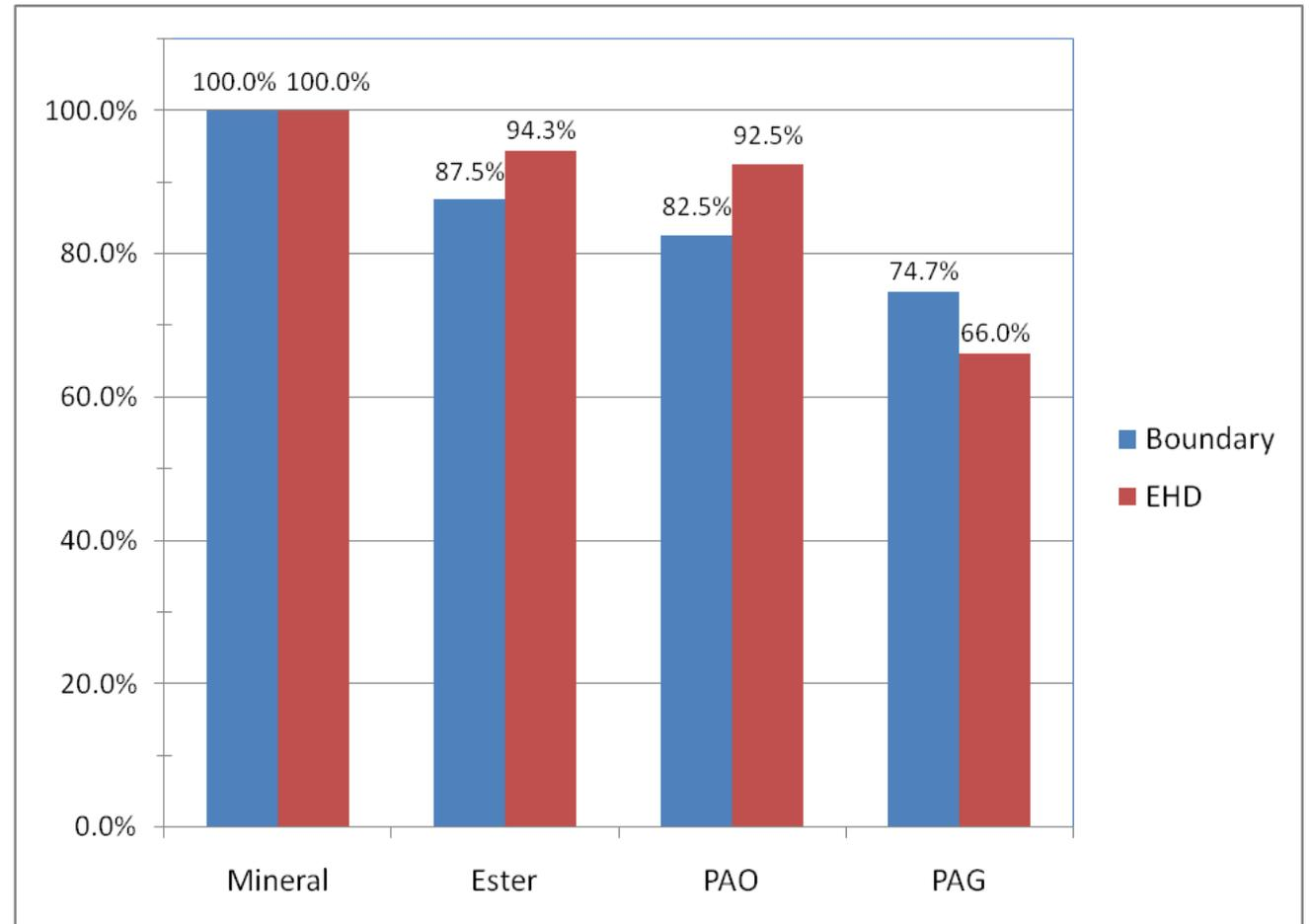
Figure 1 Boundary ( $\mu_{bl}$ ) and EHD ( $\mu_{EHL}$ ) coefficient of friction for bearings
