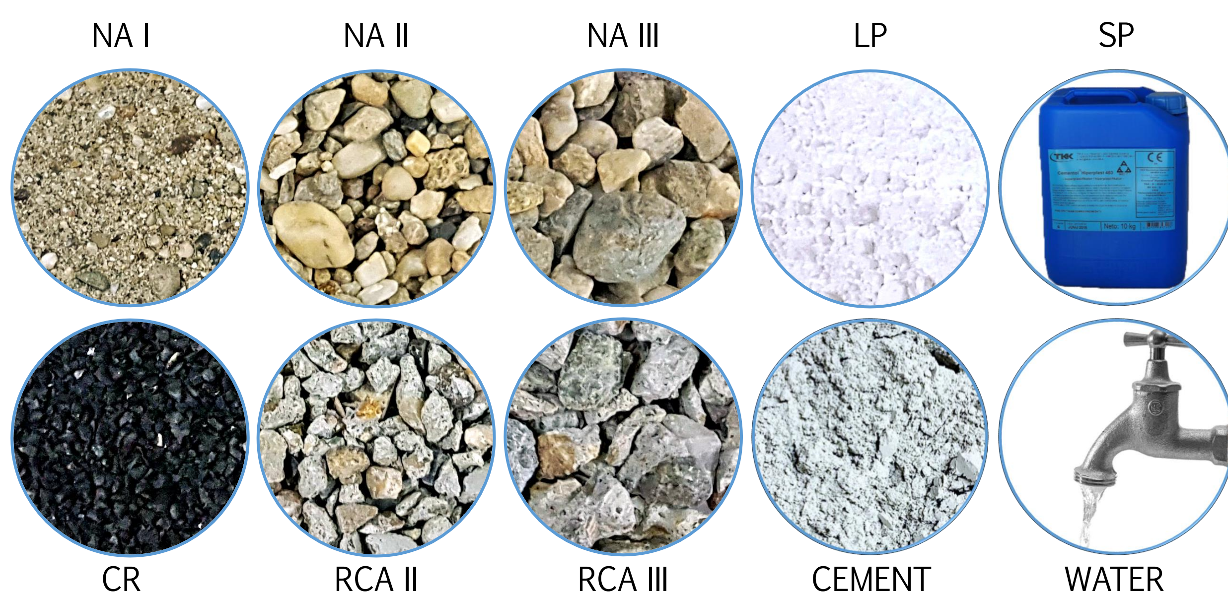
Figure 1: SCC components used in this research – NA fractions I, II and III, untreated CR and RCA fractions II and III, limestone powder (LP), portland-composite cement CEM II/A-M(S-L)42,5R, superplasticizer (SP) and water from the city water-works
